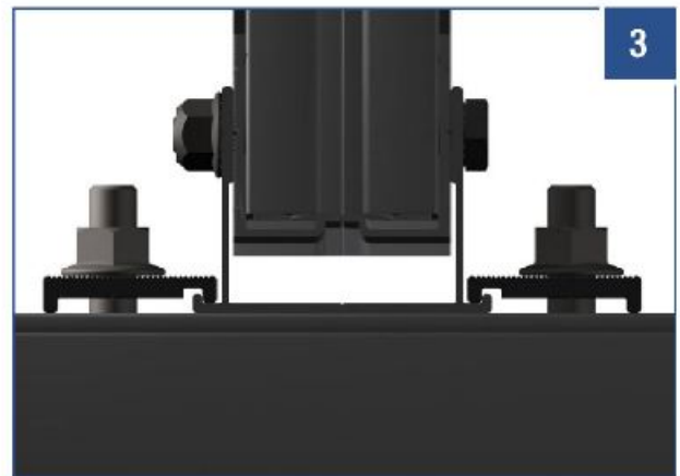
Then lay the mounting disk 9785 loosely to the threaded neck and tighten using a stop nut 985 A2/A4 M8 or a lock nut 9345 A2/A4 M8. (torque 14-16 Nm)
