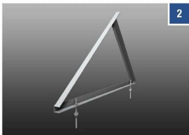
FIG. 2: Should the mounting points on the rafters, taking account of the statics calculation of the triangle casing lie at the very best, the mounting system can be installed directly to the stair bolts without using the appertaining angle.
