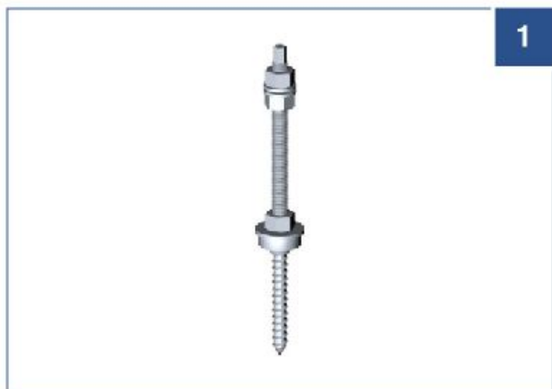
FIG. 1 Stair bolts When roofing is of corrugated sheeting or trapezoidal metal plating, stair bolts can be used. This is possible in the case of inclined roofs up to a max. 20° roof incline
