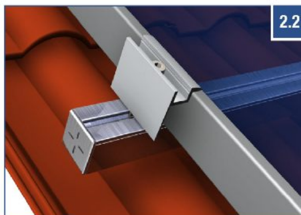
FIG. 2.1: Swivel the slot nut into the upper rail and click together. Screw the terminal clamp with the appertaining screw (each depending on module height) into the slot nut. Alternatively, click the click element into the upper duct of the rail and tighten (torque up to a max. 18 Nm depending on module manufacturer.) A cover may be used to close off the form. (FIG 2.2)
